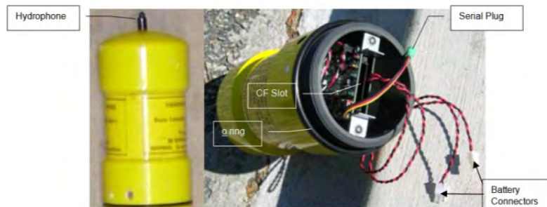
Figure 2.10. Side (Left) and Bottom (Right) Views of an Autonomous Node Top
