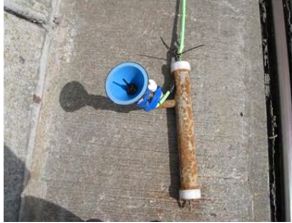
Figure 2.9. Trolleys Used to Deploy Hydrophones at The Dalles Dam Powerhouse and Spillway, 2010. A 4-in.-diameter trolley with hydrophone for deploying in slotted pipes on powerhouse and spillway piers. Each trolley had a steel arm to support a hydrophone that was surrounded by a plastic cone lined with anechoic material to prevent sound reception from a downstream direction.
